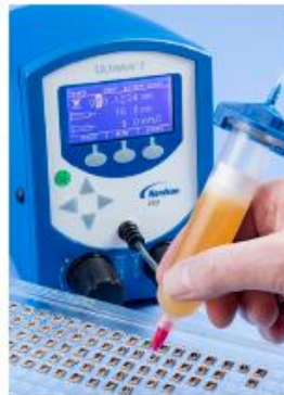
Dispensing flux onto electronic components.
