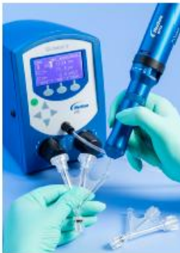
Dispensing adhesive onto medical components with HPx™ tool.
